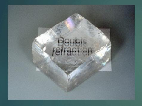
Birefringence, or double refraction, is the decomposition of a ray of light into two rays when it passes through anisotropic materials
